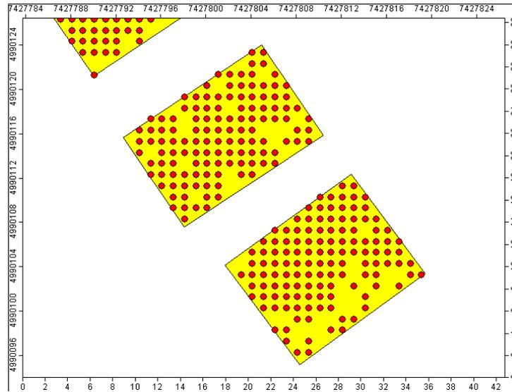
Fig 2. Cloud of remaining points after filtering for each building. Final DSM is created from the points.
