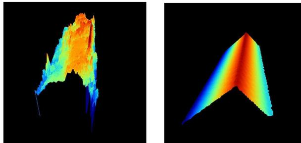
Fig. 1. An example of raw DSM of the 2-plane roof used in the experiment (left) and final 3D model of 2-planes roof (right)
